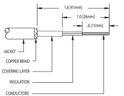
**5.** Using a very sharp, fine bladed knife (such as a utility knife or box cutter), split the insulation of the two heating conductors back to the covering layer.
