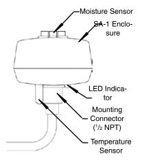
Easy Heat's SA-1 is a sensible solution for economical and effective control for powering heating cables in snow and ice melting applications. Water resistant, the SA-1 operates when snow or freezing rain conditions exist, and can regulate cable operation in sidewalks, driveways, parking garage entrances or drive-through areas — in both residential and commercial settings.
