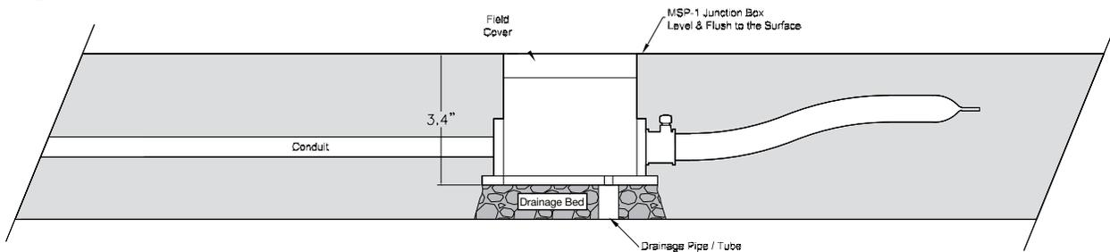
Figure 3 - MSP-1 Junction Box Installation, Plan View
