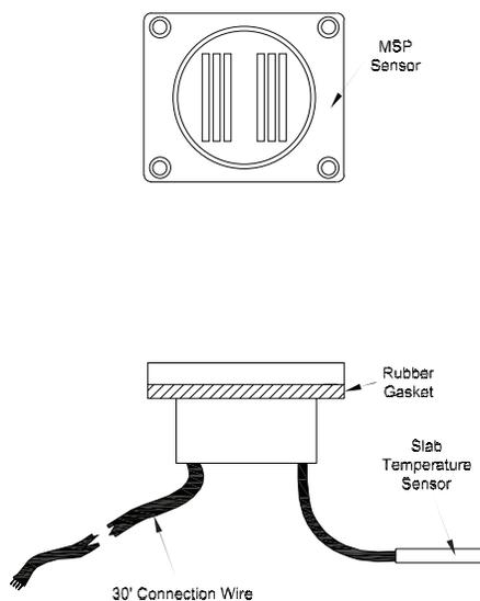
The main components of the MSG-1 are shown in Fig.1.
