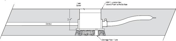
Figure 3 - MSP-1 Junction Box Installation, Plan View
